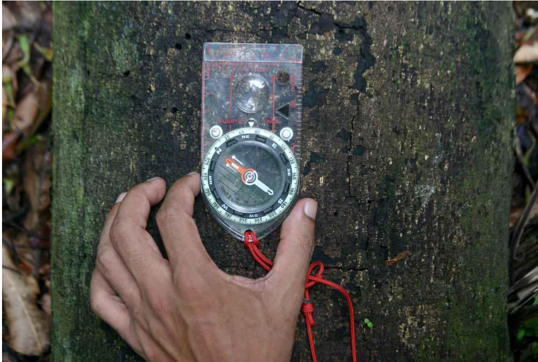
Photo 4. The orientation of a piece of coarse woody debris is assessed by placing the compass so that the compass points from the larger to the smaller end of the piece (for this model compass, the direction is indicated by the two narrow red arrows above the dial). Then turn the dial so that North points to magnetic North (here the red end of the needle between the white marks) and read the direction (degrees indicated at the white triangle above).
