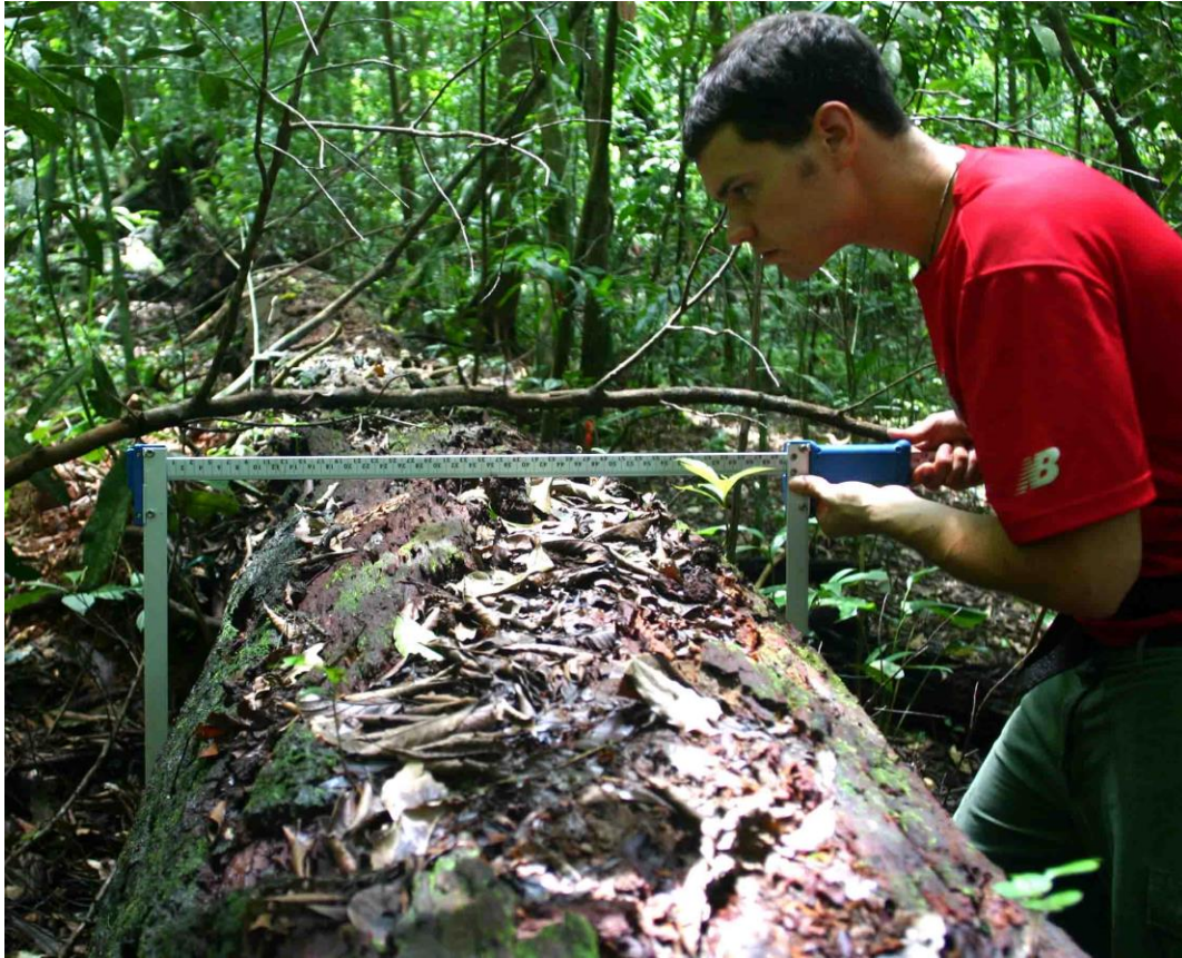
Photo 3. The diameter of a piece of coarse woody debris is measured using a large caliper. Because the two blades of the calipers bend easily, care must be taken to apply the correct amount of force so that the blades remain parallel. (This can be practiced by measuring diameters of small objects such as sticks, placing them at various positions between the blades while observing whether the blades are parallel.)
