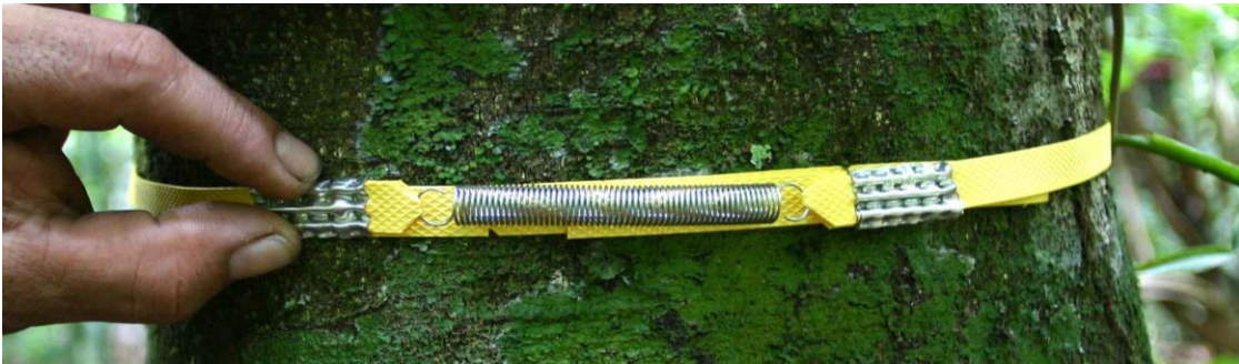
Figure 6: Plastic dendrometer installed on a tree. Note that the seals look quite different when fastened. The spring is attached between folded over parts of bands, with both ends of each fold cut. The notch in the lower band and the free end of the upper band are both visible beneath the spring.
