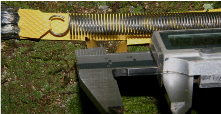
Figure 7: The caliper measurement is made from the notch on the lower band to the free end of the upper band.
