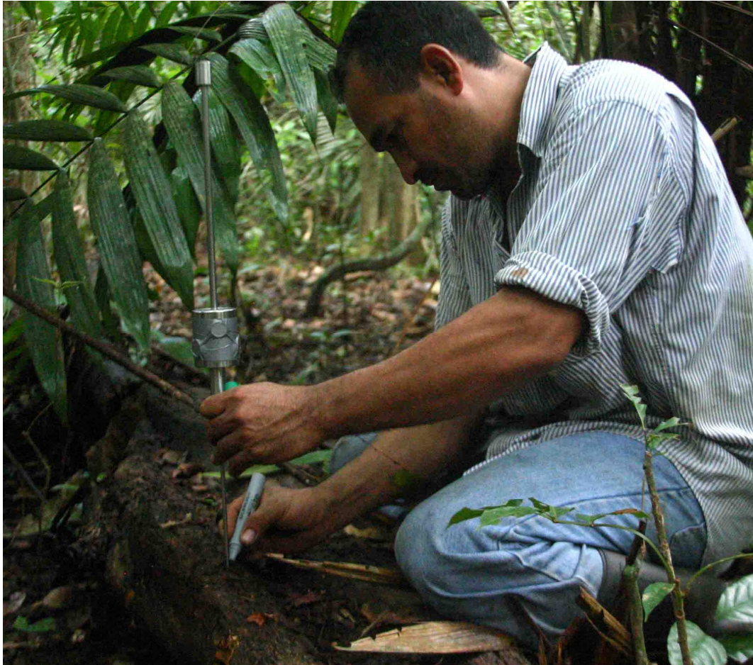
Photo 2. The hardness is assessed with a penetrometer. A nonpermanent marker is used to mark the depth of penetration before removing the instrument from the woody debris.
