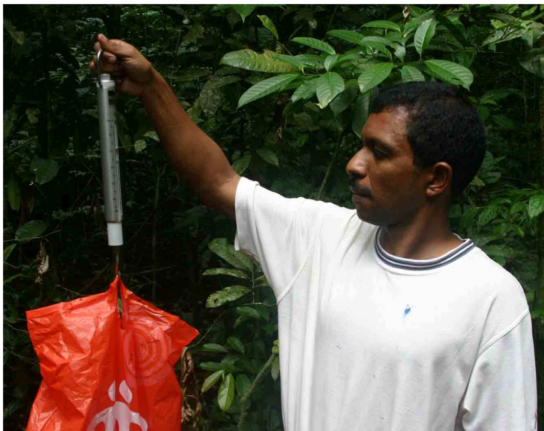
Photo 4. The samples of coarse woody debris are weighed in the field with a portable balance (model in the photo different from the one mentioned in “Materials Needed in Field”).
