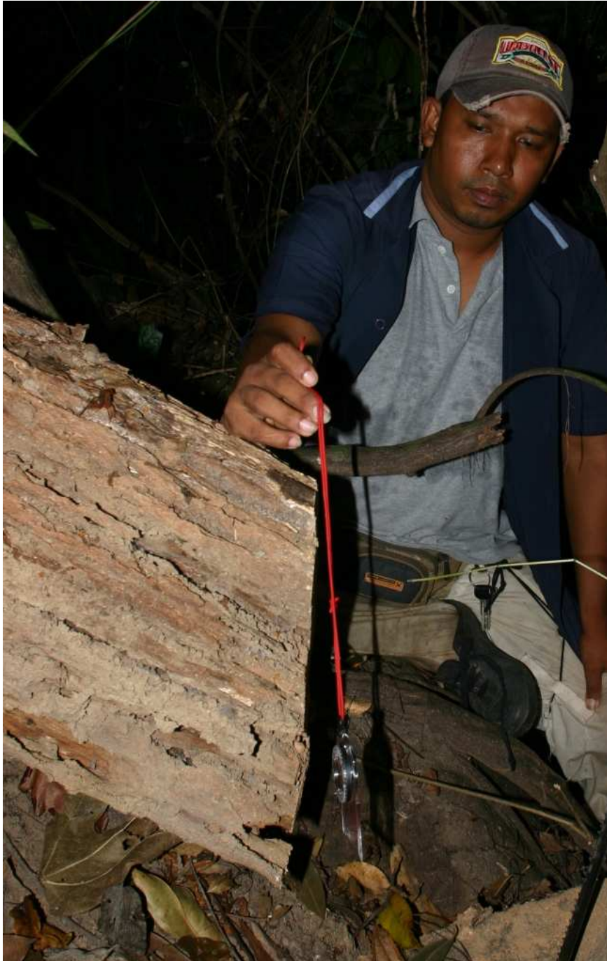
Photo 3. It is important to check with a hanging object (e.g. compass) that the cuts are vertical. For example in the photo the cut was not vertical and therefore cause underestimation.
