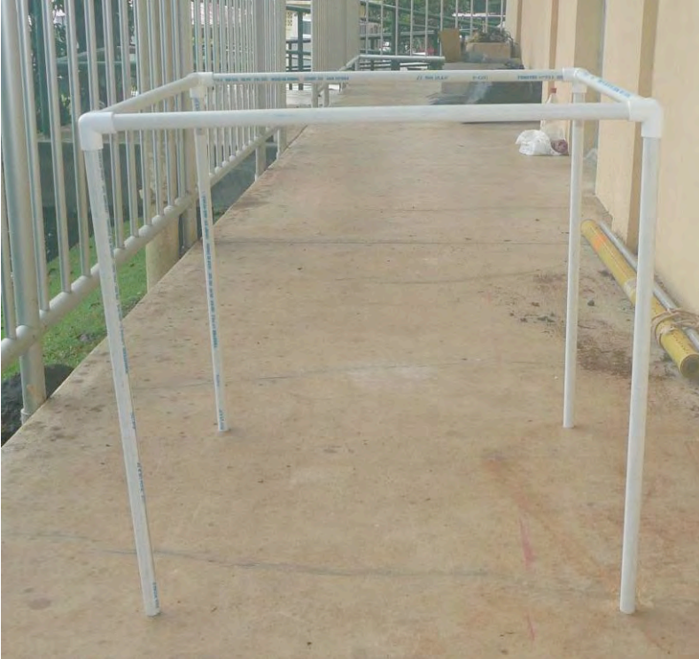
Figure 3. The alternative aboveground trap design, which requires “right angle outs” at the trap corners.
