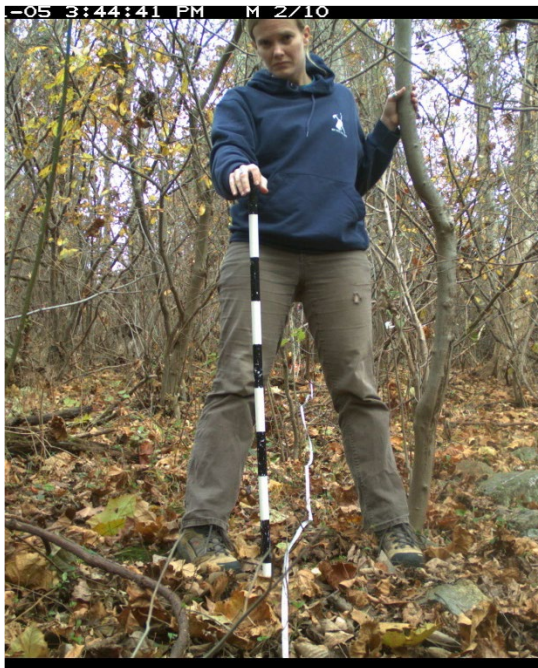
Figure 4. A camera trap picture of camera calibration with a black-and-white pole. This calibration is done to aid 3D image recognition by computers.
