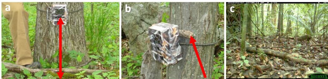
Figure 3. Alignment of the camera trap. (a) The lens of the camera is exactly 50 cm from the ground. (b) Sticks are placed between tree and camera, if necessary, to tilt the camera, so that its view is exactly parallel to the ground; downhill in this example. (c) The “view” of a properly installed camera.
