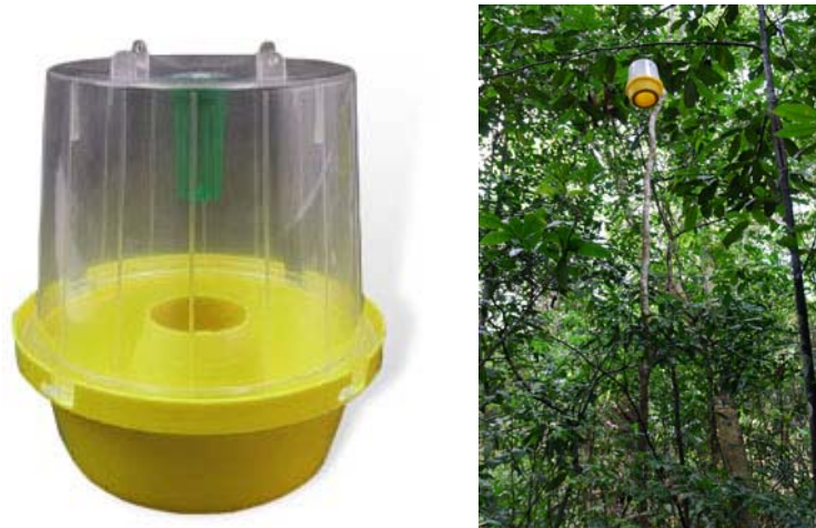
Fig.5. Detail of McPhail trap (ca 20cm tall, left) and as set up in the field (right).
